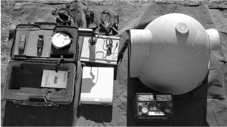
Figure 1. The video system used for monitoring above-ground ferret activity in southwestern South Dakota, June through October 2006. The system included, from left to right, carrying case with cables and viewer, video cassette recorder, video camera, igloo-style dog house, and 12V battery.
